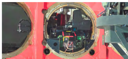
SHARK-VIS mounted at the LBTI bent Gregorian focal station – the instrument is in the black L-shaped enclosure in the upper right quadrant.
