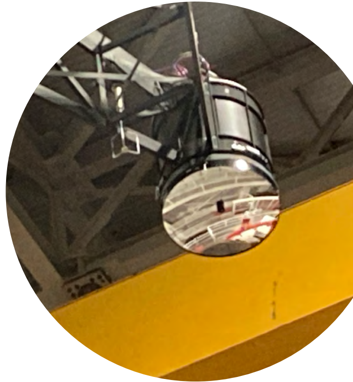
SX adaptive secondary mirror with recoated thin shell, on the telescope in September 2023.
